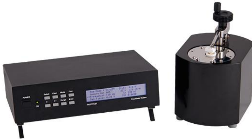
Figure A-1. Commercial Berlincourt d_{33} PiezoMeter which measures the d_{33} of a sample by clamping the sample and subjecting it to a low frequency force to an accuracy of \pm 2\% .
