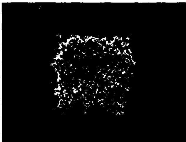
**Figure 2.3:** Scanning electron micrograph showing a 50 by 50 $\mu$ m pixel patterned using HCl etching solution; the HCl has quickly attacked the PZT grain boundaries
