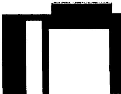
7) First DRIE step to define beam or diaphragm thickness
