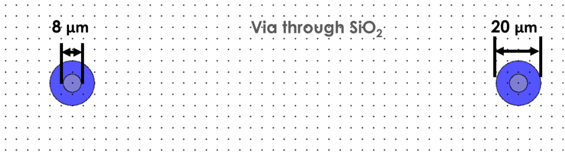
Figure 6-8: Pattern of the 8\text{ }\mu\text{m} diameter wet etch vias over the top electrodes.
