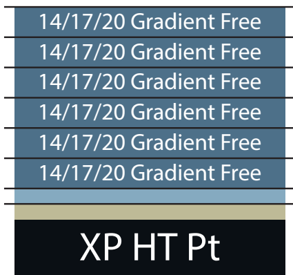
Figure 4.6: Schematics of the layer sequences utilized to deposit niobium doped gradient free thick films.
