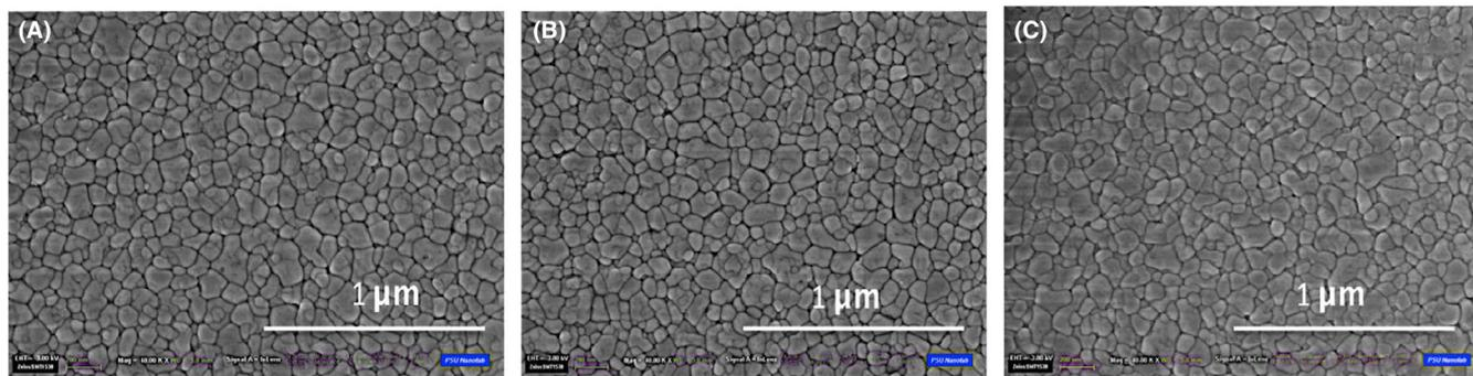
**FIGURE 3** Top surface SEM images of PZT films annealed at distinct PbO partial pressures: (A) low PbO partial pressure (yellow line in Figure 2), (B) intermediate PbO partial pressure, and (C) high PbO partial pressure (red line in Figure 2). FESEM images were taken after patterning of Pt top electrodes
