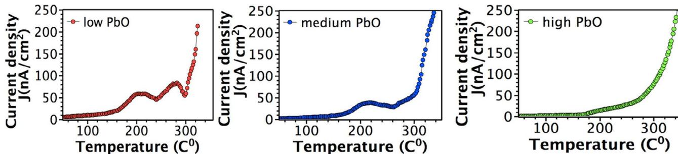
**FIGURE 7** TSDC spectra in PZT films annealed under low, medium, and high PbO activities. TSDC data were attained after degrading the films under an electric field of 275 kV/cm at 180°C for 12 h. A 6°/min heating rate was used to attain TSDC peaks
