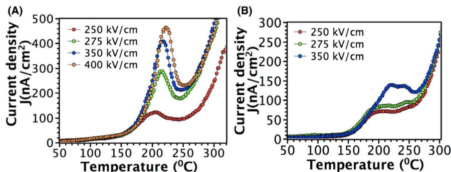
**FIGURE 5** Estimation of activation energies for TSDC peaks arising from 2 mol% Mn-doped PZT films using three distinct methods: (A) initial rise model, (B) FWHM method, and (C) different heating rate ( $6$ – $10^\circ\text{C}/\text{min}$ ). The films were degraded under an electric field of 275 kV/cm at  $180^\circ\text{C}$  for 12 h
