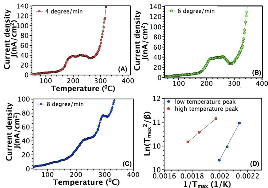
**FIGURE 6** (A–C) Thermally stimulated depolarization current data of 2% Nb-doped PZT films for different heating rates (4 and 8°/min), (D) Estimation of activation energies for the low- and high-temperature TSDC peaks using heating rate method. The films were degraded at 180°C under an electric field of 350 kV/cm for 12 h
