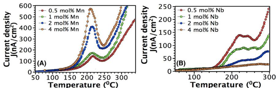
**FIGURE 8** Evolution of TSDC peaks in degraded PZT films with increasing (A) acceptor (Mn) dopant concentration, and (B) donor (Nb) dopant concentration. The films were degraded at 180°C under an electric field of 350 kV/cm for 12 h. TSDC data were obtained using a ramp rate of 8°C/min
