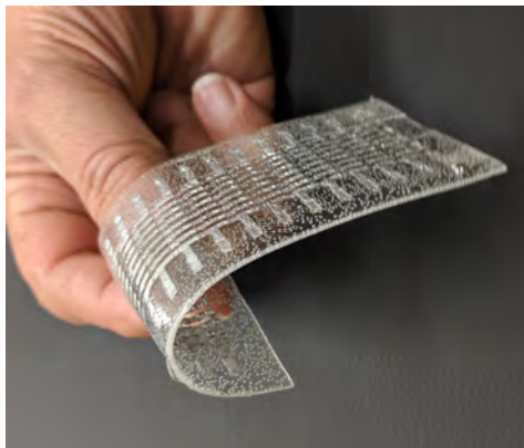
Figure 3. Flexible TEG array made from liquid metal interconnects and flexible polymers
