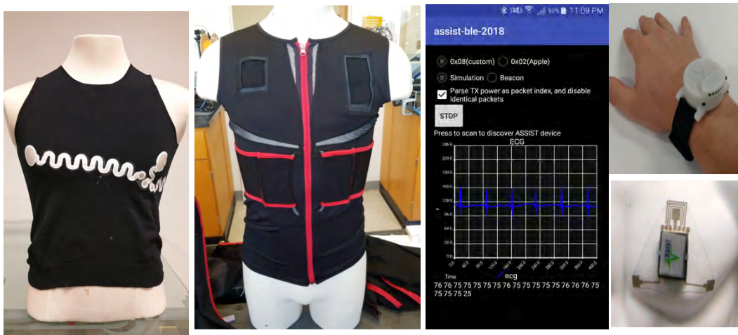
Figure 11: (a) ink jet printed Ag/AgCl metal electrodes on textiles, (b) fully functional A-Fib shirt indicating location for harvesters and antenna, (c) typical R-R measurements, (d) environmental detection watch and (e) ECG/hydration patch
