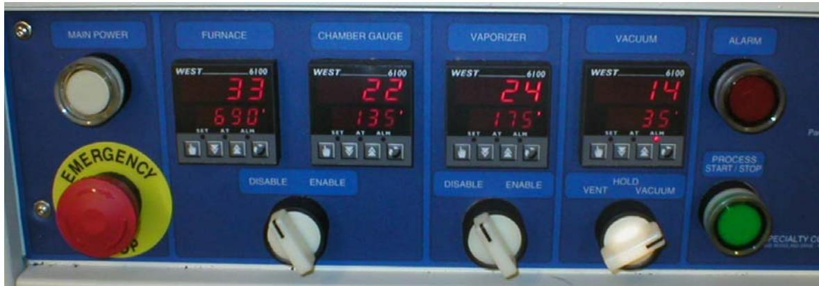
**Control Panel on the Parylene Deposition System**
