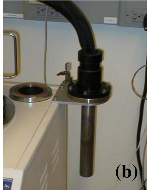
**Cold finger (a) pumped down and (b) in the outer holder.**
