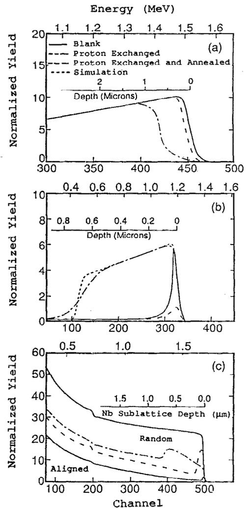
FIG. 1. Li depth profiles (a) H depth profiles (b) and ion channeling results (c) for *X*-cut  $\text{LiNbO}_3$  blank, after proton exchange in benzoic acid at 180 °C for 1 h, and after thermal annealing in air at 350 °C for 10 h.
