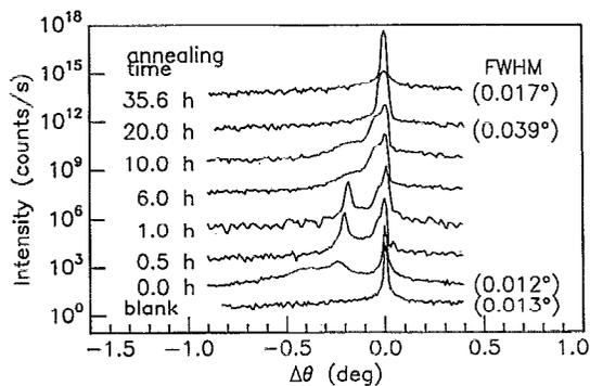
FIG. 2. X-ray rocking curve analysis for *X*-cut LiNbO<sub>3</sub> after exchange in benzoic acid at 180 °C for 1 h and thermal annealing in air at 350 °C for various times.
