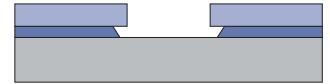
4. Develop resist and PMGI. PMGI develops isotropically, creating a bi-layer reentrant sidewall profile.
