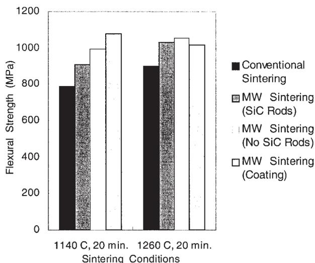
**9 Histogram showing comparison of flexural strength for conventional and microwave sintering for two different sintering conditions**
