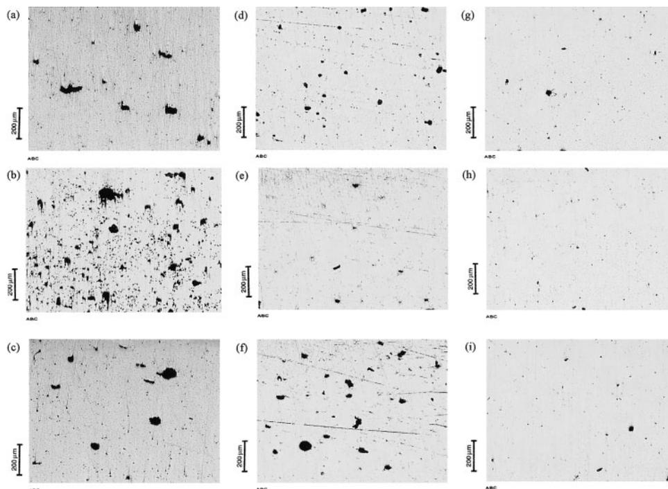
**10** Optical micrographs showing porosity distribution of conventional sintered (*a–c*), microwave sintered with SiC susceptor (*d–f*), and microwave sintered with coating susceptor (*g–i*) unetched samples. Centre micrographs (*b, e, h*) represent core, while rest of micrographs represent edges of copper steel MOR bar samples
