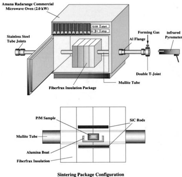
1 Schematic diagram of microwave sintering set up
