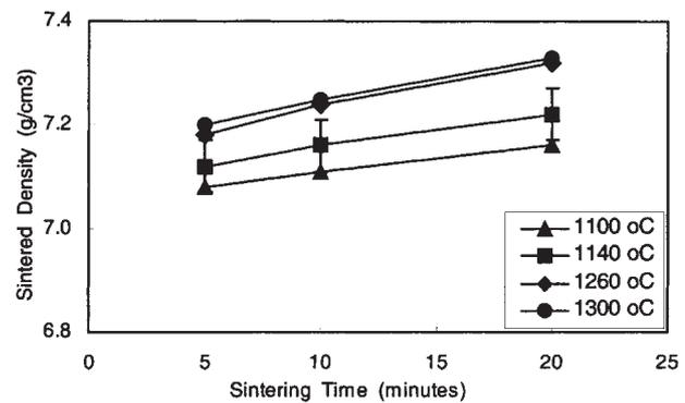
4 Sintered density of copper steel MOR bar samples sintered in microwave system using SiC susceptor, as function of sintering for different sintering temperatures
