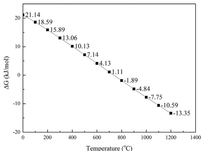
Fig. 3. Ellingham diagram for the conversion of  $\alpha$  to  $\beta$ -spodumene.  $\Delta G$  values were calculated in HSC Chemistry-6.0 [35].
