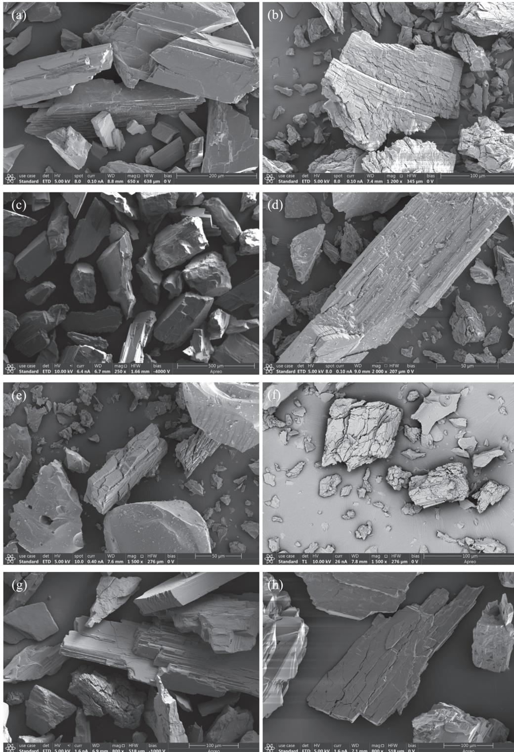
**Fig. 5.** SEM images of (a) spodumene concentrate, and calcined spodumene via (b) conventional heating at 1100 °C, and microwave heating at (c) 0.5 kW, (d) 1.0 kW, (e) 1.5 kW, (f) 2.0 kW, (g) 2.5 kW, and (h) 3.0 kW powers.
