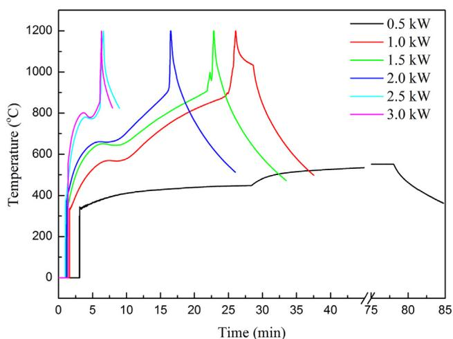
Fig. 2. Measured spodumene temperature profiles under different microwave powers (0.5–3 kW).
