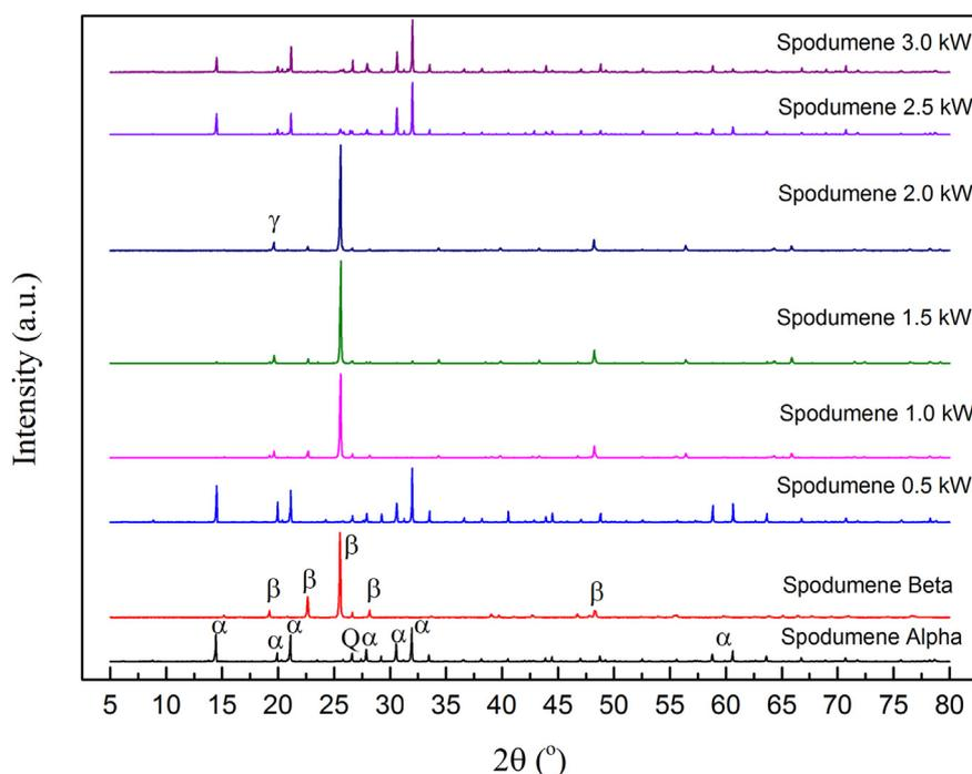
Fig. 4. XRD patterns of the spodumene concentrate (i.e., spodumene Alpha) and calcined concentrate samples via conventional heating (i.e., Spodumene Beta) and hybrid microwave heating at different microwave powers of 0.5–3.0 kW.  $\alpha$ — $\alpha$ -spodumene;  $\beta$ — $\beta$ -spodumene;  $\gamma$ — $\gamma$ -spodumene; Q—quartz.
