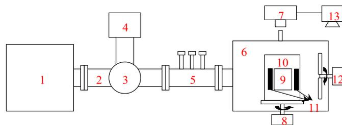
**Fig. 1.** Schematic of the microwave system (multimode, 2.45 GHz, 6 kW).
