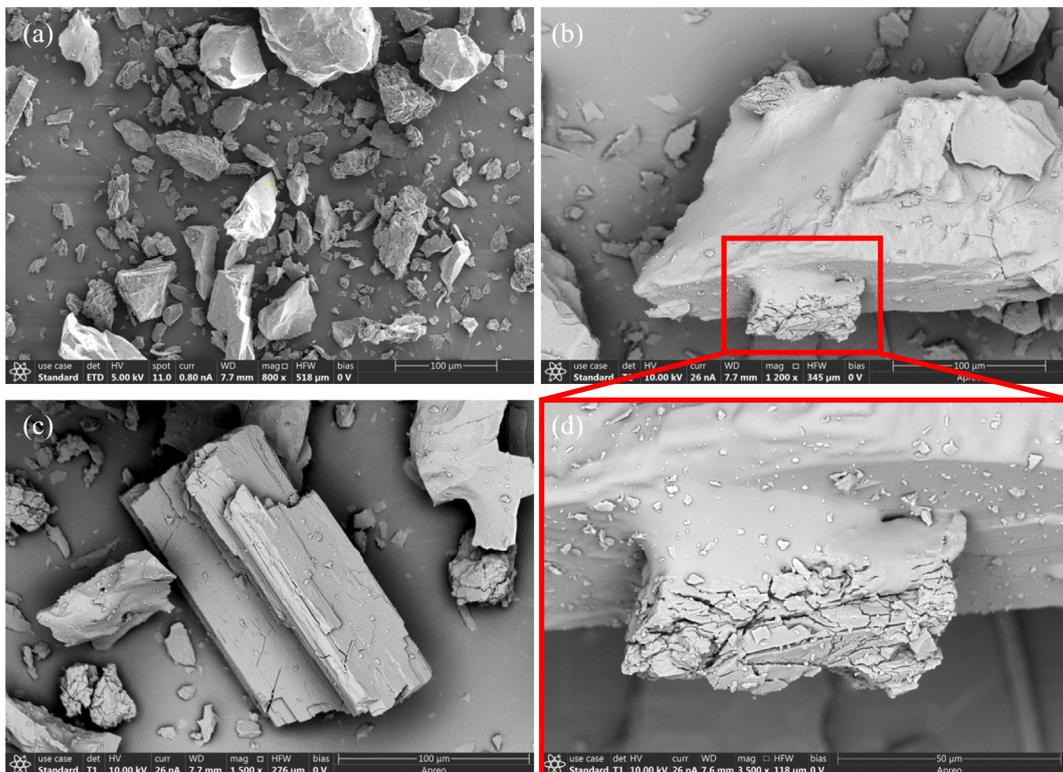
Fig. 6. SEM images of microwave-assisted calcined spodumene particles with melted parts on the surface at the microwave powers of (a) 1.0 kW, (b) 1.5 kW, (c) 2.0 kW, and (d) inset of (b) at a higher magnification.
