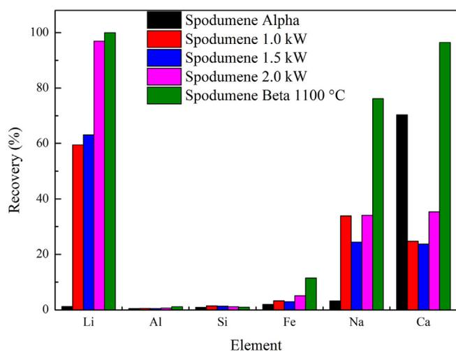
Fig. 7. Comparison of leaching recovery of major elements from the spodumene calcined via microwave and conventional heating methods.
