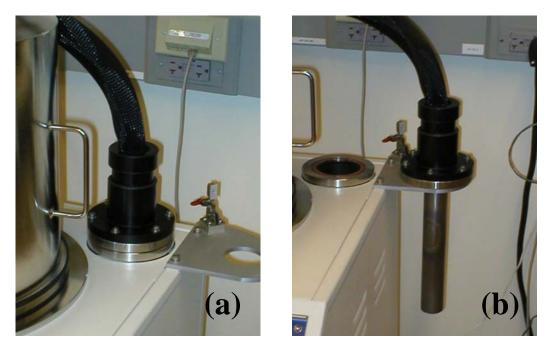
Cold finger (a) pumped down and (b) in the outer holder.
