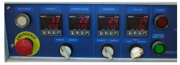
**Control Panel on the Parylene Deposition System**
