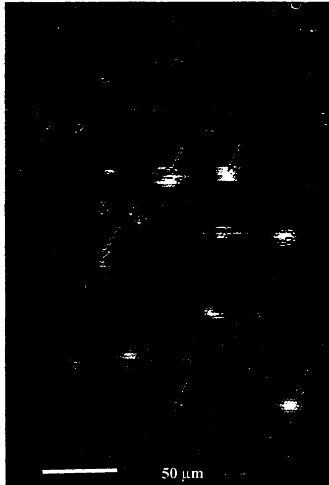
Figure 5.9. Image quality map obtained using OIM shows the morphology of the grains. Light gray areas (marked by red arrows) at the center of large grains are the template particles.
