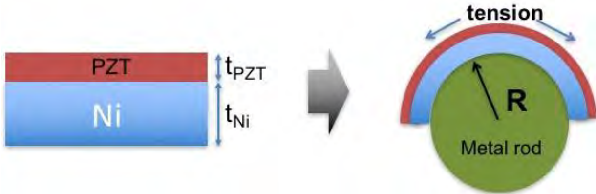
Figure 8-2. Schematic of cross-section of PZT film bent around a metal rod.
