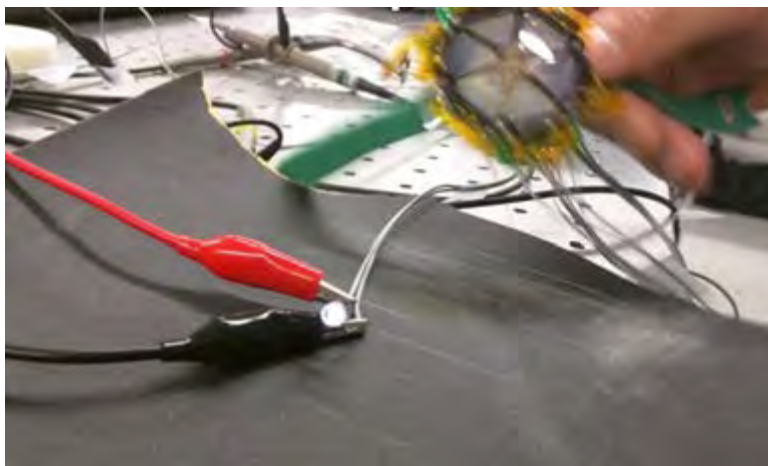
Figure 7-28. Capture of a video showing flashing of an LED through one unimorph beam by hand shaking the harvester.
