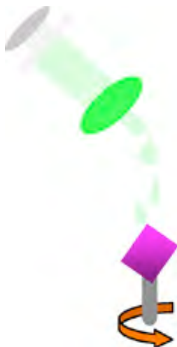
Figure 3.3: Illustration of spin coating
