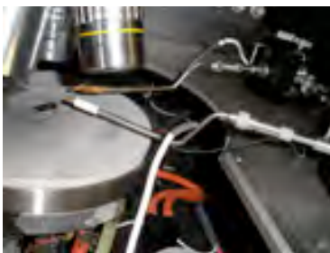
Figure 3.6: A two-probe setup used for TCR measurements
