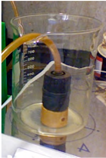
Figure 3.11: Fixture to hold tubing in the solution during the deposition
