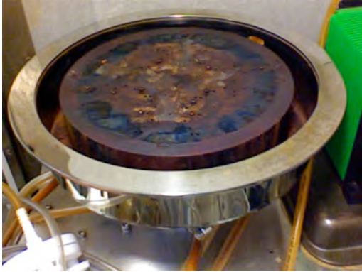
Figure 3.9: Heated substrate holder in spin spray system
