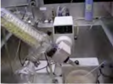
Figure 3.2: LABCONCO rotary evaporator and silicone oil bath
