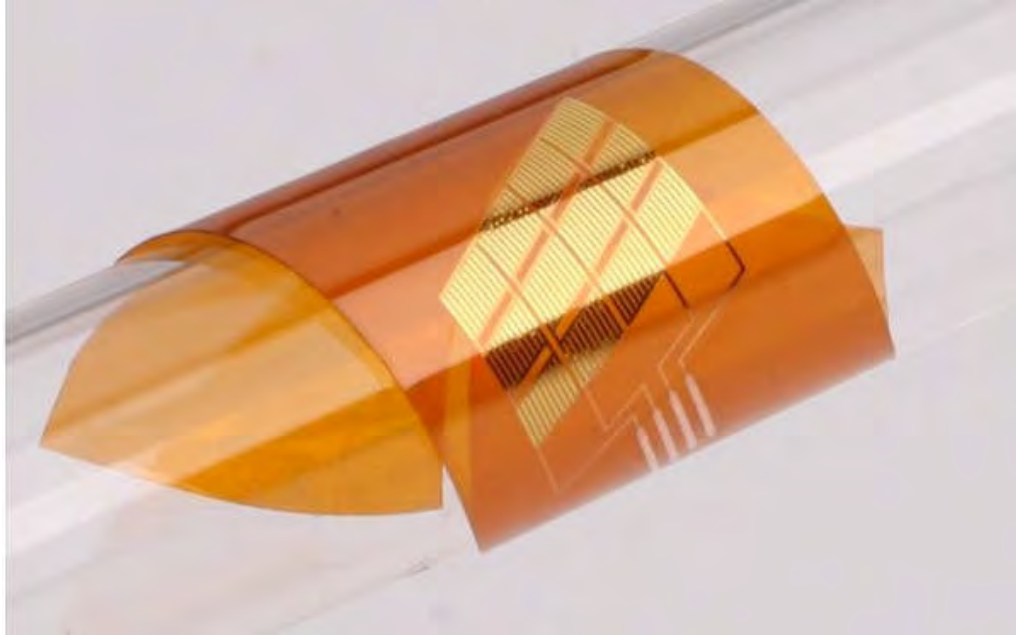
Figure 1-1 Flexible mechanical energy harvesters (MEHs) containing PZT nanoribbons for energy harvesting from organs (from Ref. [19]). Here, transfer printing was used for the heterogeneous integration.
