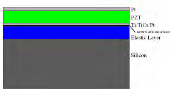
Figure 3.5: Depiction of the starting wafer composite thin film stack (Si/elastic layer/Ti/TiO 2 /Pt/TiO 2 /PZT/Pt).
