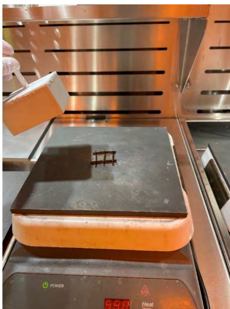
Figure D1: Experimental setup for pyrolyzing both sides of the sample after each dip. Instead of placing the substrate directly on the hotplate, a stainless-steel bracket was created to “prop” the sample up one millimeter above the hotplate surface. A ceramic box was placed over the sample on each hotplate to improve temperature uniformity around the entire sample.
