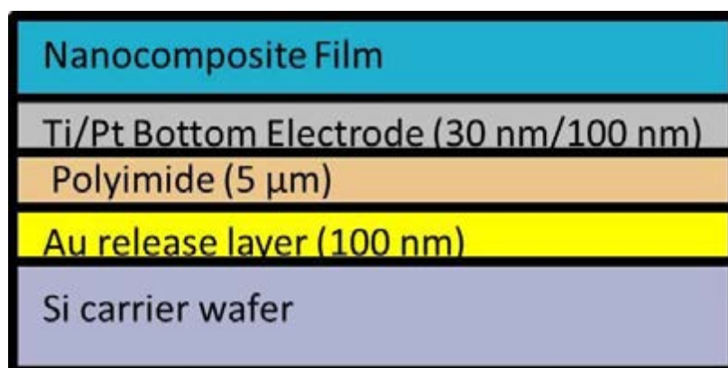
Figure 3-2. A schematic of the multilayer stack used to fabricate nanocomposite bismuth zinc niobate tantalate thin films on flexible polyimide substrates.
