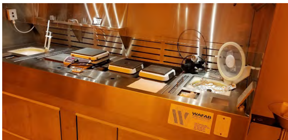
Figure 3-4: Films were deposited in the spin system in a PSU Nanofabrication facility with a controlled atmosphere and at 21% relative humidity.
