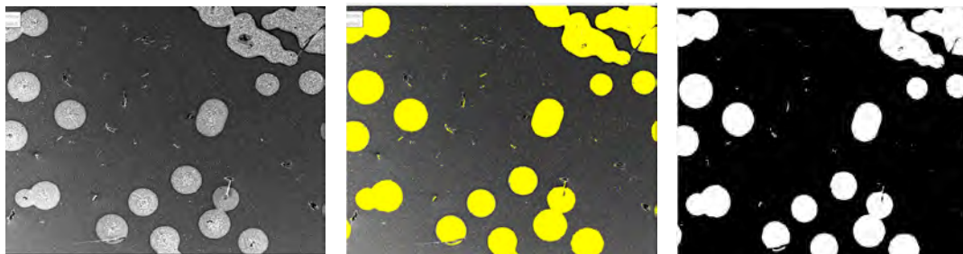
Figure A-12: Microscopy of a partially crystallized KNN film without a sonicating IPA bath prior to deposition. The dark area is the amorphous matrix. The brighter areas are the crystalline rosettes. The raw FESEM image (left) was segmented using adaptive image segmentation or the graph-cut method (middle) to generate a binary image (right). Small amounts of debris are falsely recognized as crystalline KNN.
