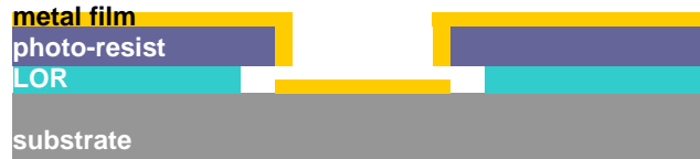
Figure 3.7 Re-entrant profile created with LOR resist in bi-layer lift-off process used for IDE.
