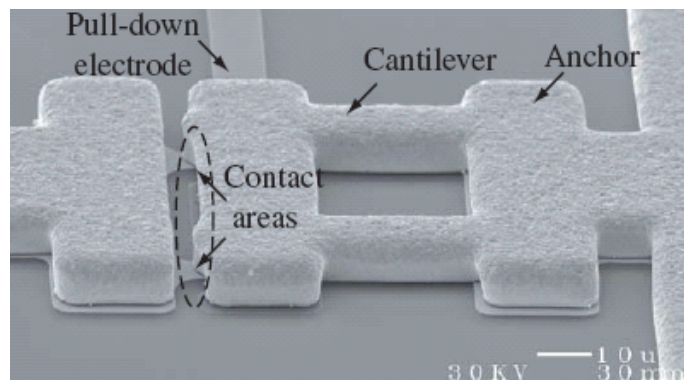
Figure 1.7 SEM image of the Northeastern University electrostatic cantilever switch. 18
