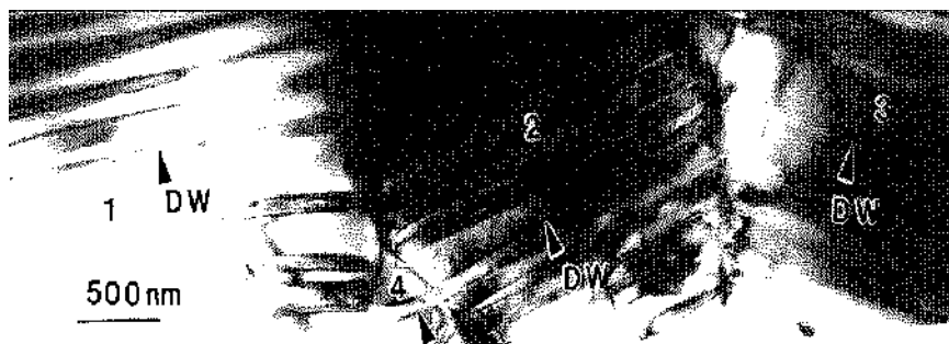
Figure 5- 22: An example of transgranular coupling in a PZT ceramic. DW denotes domain wall [49]
