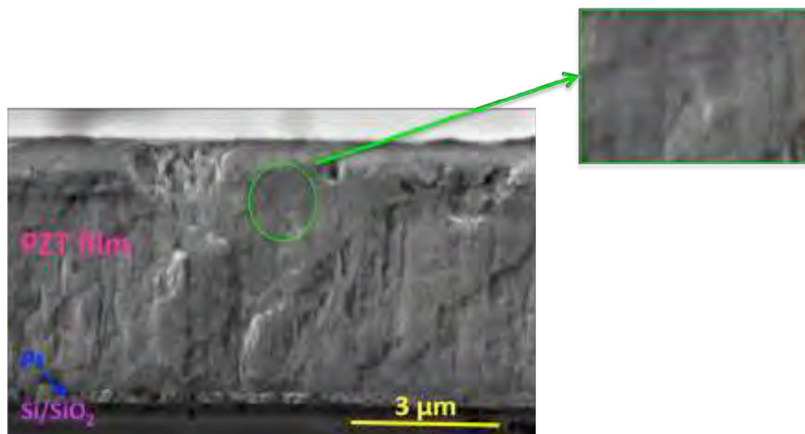
Figure 3- 5: \text{Pb}(\text{Zr}_{0.52}\text{Ti}_{0.48})\text{O}_3 films with optimized condition, 250°C, 1 min and 400°C, 1 min and RTA 700°C, 1 min, heating rate 4°C/s
