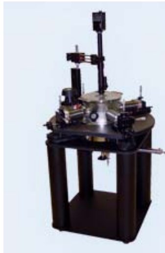
Figure 3.13: A picture of the Desert cryogenic probe station used in this work.
