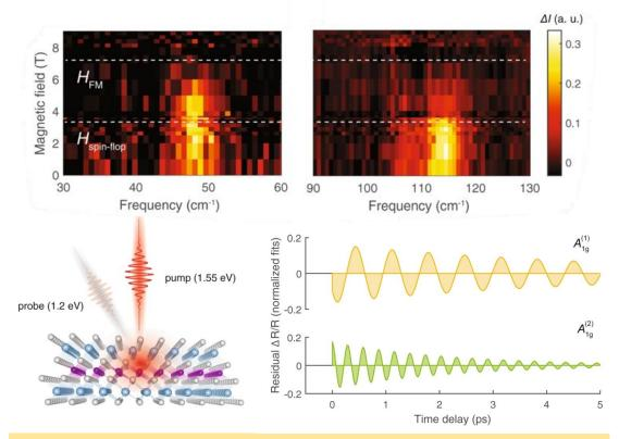
Contour plots of the difference of Raman spectra upon subtracting the 9 T spectrum, as a function of magnetic field. The dotted lines denote the ferromagnetic and spin-flop critical fields (top panels). Schematic of pump-probe measurement (bottom left). Individual decaying sinusoidal components corresponding to the  $A_{1q}^{(1)}$  and  $A_{1q}^{(2)}$  phonons, respectively (bottom right).
