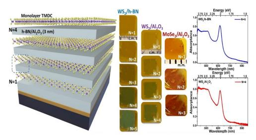
Intense, narrow band absorption demonstrated in optical dispersion engineered TMDC/dielectric superlattices enabled by the availability of wafer-scale 2D monolayers.
