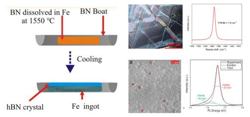
Schematic illustration of hBN crystal growth using the single component Fe flux method.
