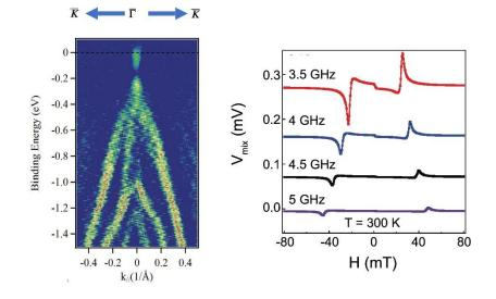
(Left panel) Second-derivative ARPES spectrum from a 30 nm thick (112) oriented  $Cd_3As_2$  film grown by MBE on GaSb/GaAs (111). (Right panel) Measurements of ST-FMR in a  $Cd_3As_2$  (40 nm)/Ni<sub>0.8</sub>Fe<sub>0.2</sub> (30 nm) heterostructure. All data are taken at T = 300 K.
