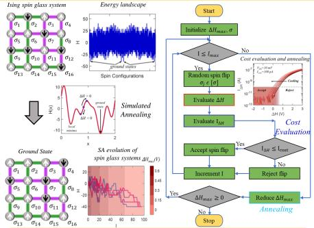
SA algorithm is used to identify the ground state of a Ising spin glass system. In the SA flowchart, evaluation of change in energy ( $\Delta$ H), cost evaluation and annealing are performed with the aid of MoS<sub>2</sub> FETs (MoS<sub>2</sub> obtained from 2DCC).
