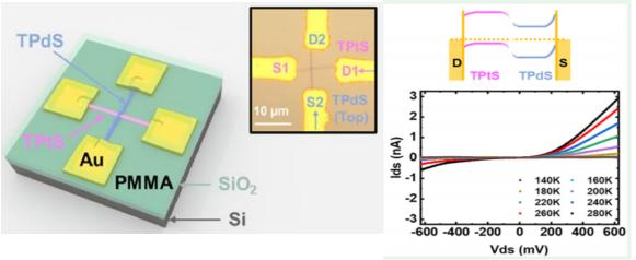
Left panel: Schematic diagram of a nanoscale crossed junction between perpendicularly stacked n-type  $Ta_2Pt_3Se_8$  (TPtS) and p-type  $Ta_2Pd_3Se_8$ (TPdS) nanowires. Inset: Optical micrograph of a typical device. S and D indicate the source and drain electrodes, respectively.
