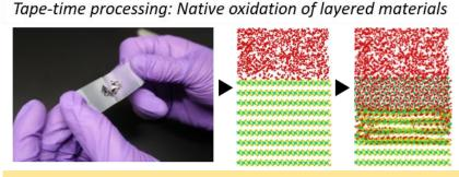
Experiments reveal time-dependent oxide growth after tape exfoliation. Simulations reveal atomic mechanisms that promote and suppress oxidation.
