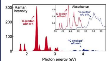
The so-called "C exciton" resonance appears very strongly in full Raman intensity calculation (red), but is much weaker in a calculation that omits excitonic effects (blue). The efficient perturbative approach used here also opens up the method to much more complex systems and high-throughput data-intensive modes of analysis.
