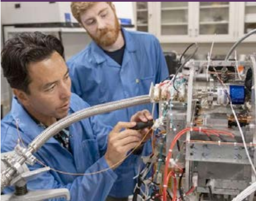
Randall McEntaffer, head of Penn State's Department of Astronomy and Astrophysics, makes adjustments to the flight electronics and power supply of the X-ray spectrometer that he and his team built for a September launch with NASA. Credit: Patrick Mansell/Penn State Creative Commons
