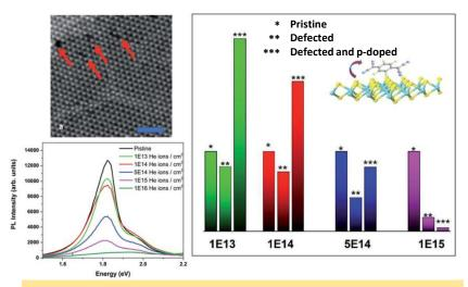
A Helium Ion Microscope was used to introduce a controlled density of sulfur vacancies in monolayer  $MoS_2$  which resulted in decreasing photoluminescence intensity. For lower defect concentrations, the introduction of a p-type dopant molecule (FATCNQ) enabled a recovery and significant enhancement of light emission.
