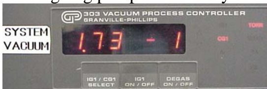
Figure 5-1: Vacuum Process Controller showing vacuum less than 200mTorr (173mTorr).
