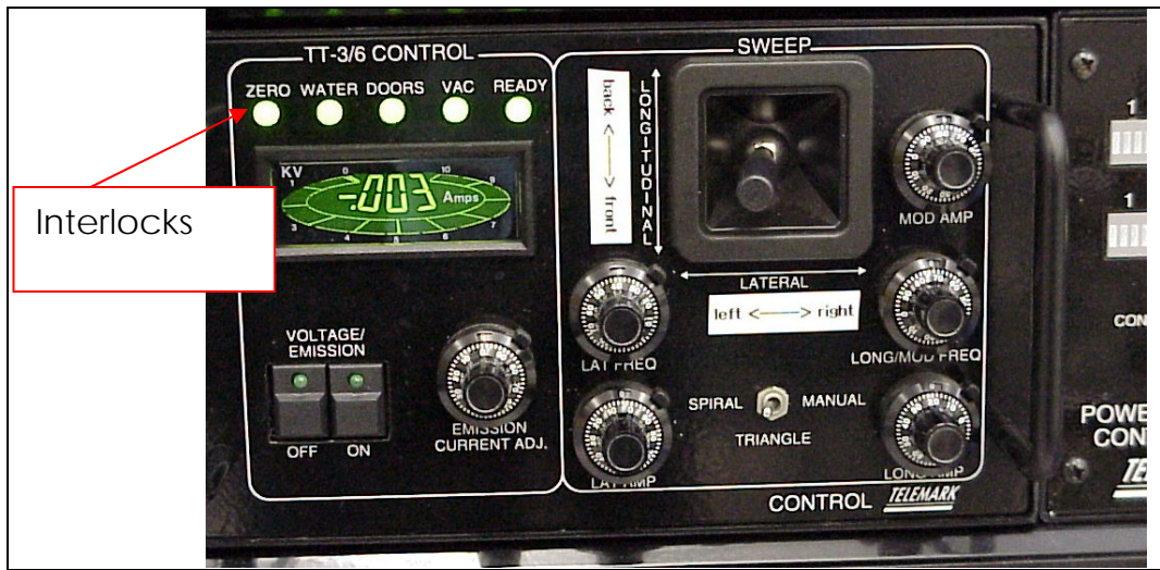
Figure 7-3: Telemark Power Controller interlocks
