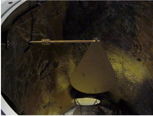
Figure 2-24: View of inside of chamber with the shutter in the down (dropped) position
