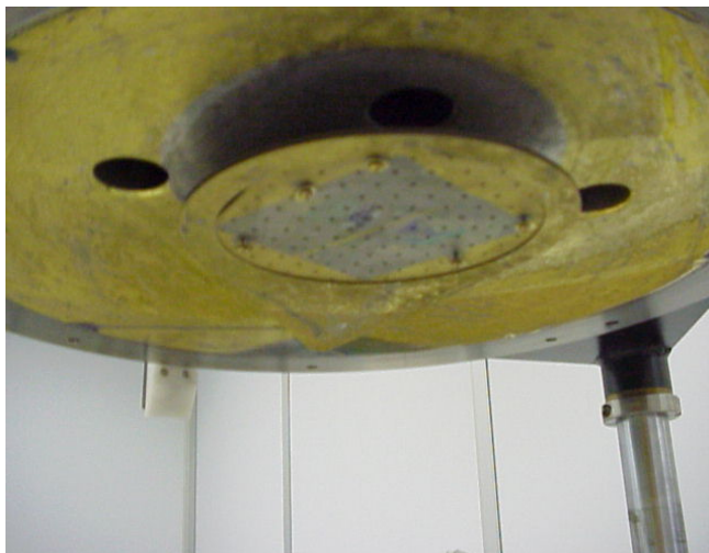
Figure 2-16: Sample state with 6" small parts holder loaded.
