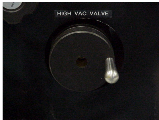
Figure 2-2: High Vacuum Valve Completely Closed
