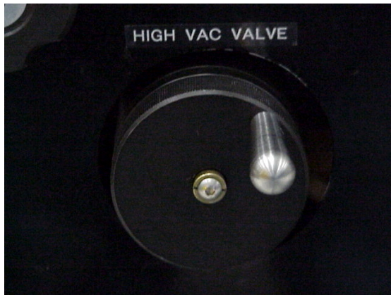
Figure 2-19: High vacuum valve fully open
