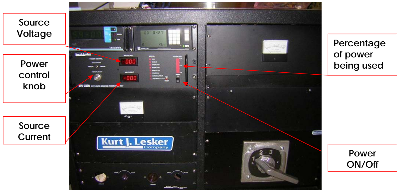
Figure 2-25: Thermal source controller
