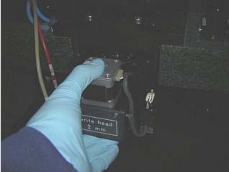
Figure 2-11: Sliding write head off of rails
