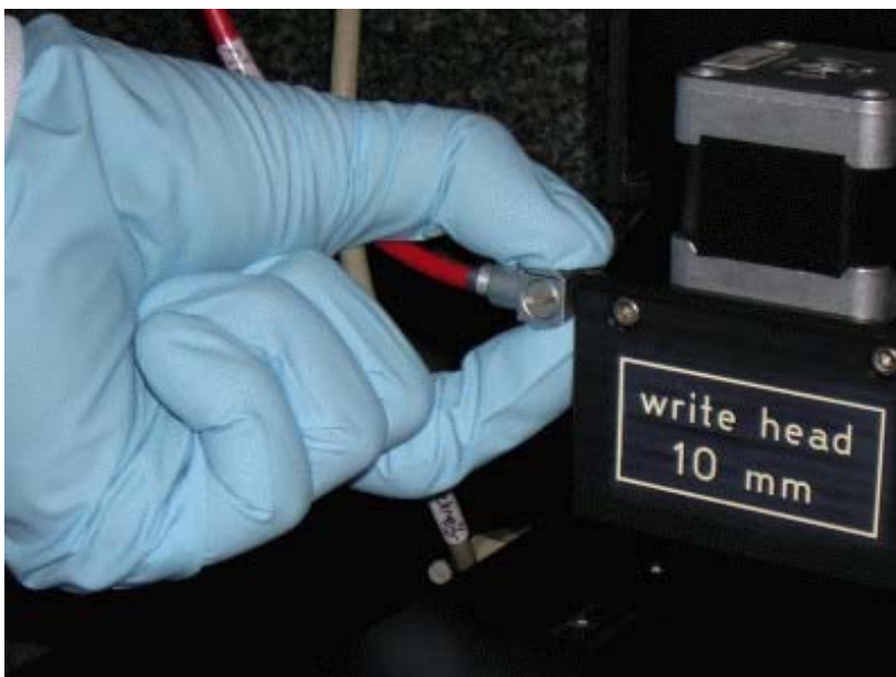
Figure 2-8: Releasing write head red coax cable by squeezing the connector
