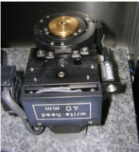
Figure 2-12: Write head stored upside down
