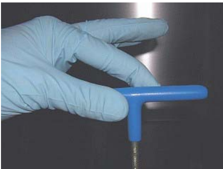
Figure 2-13: Tighten with two fingers
