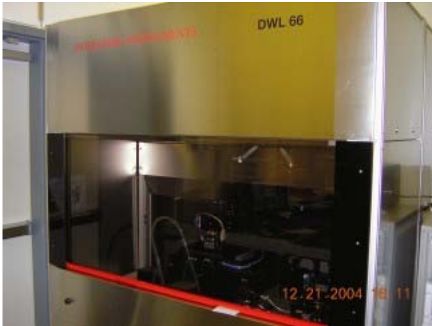
Figure 1-1: DWL 66 Main system environmental chamber contains laser optics, stage, and camera systems
