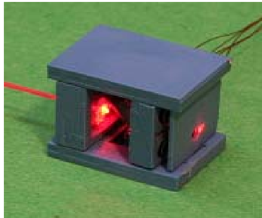
Integrated Optical Fiber Alignment Package (IFAP) with a delta-shape 2D-freedom piezoelectric ultrasonic motor. [2007 R&D 100 Award product]
